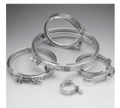
V-Band Couplings eliminate the need for cumbersome bolted flange designs and costly welded flange designs. Because V-Band Couplings can be easily assembled and disassembled, they are often used on equipment that requires frequent service or maintenance. Typical V-Band applications include Turbochargers, Diesel Aftertreatment and Exhaust Systems, Pumps, Filters and Fluid/Bulk Solids Processing Equipment.
